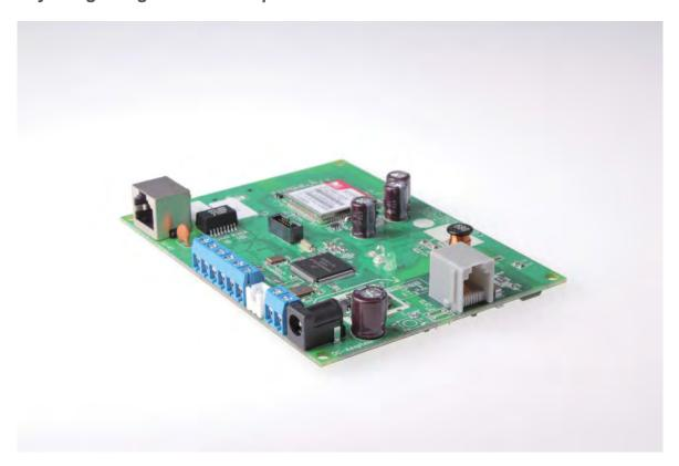
VST-1905-M1/M8/M8 EX are PSTN-to-IP/GPRS/3G Converters that switch PSTN control panels from traditional phone landlines to IP/GPRS/3G networks. The plug & play installation of this Converter series requires no replacement or dismantling of the host control panels. Any PSTN alarm panel adopting the CID reporting format can be easily adapted for IP/GPRS/3G based monitoring centers by VST-1905-M1/M8/M8 EX, which seamlessly converts PSTN CID into SIA protocol and CID over IP/GPRS/3G
